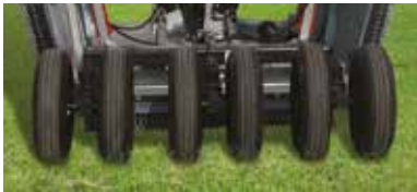
Triple Center Axles are standard on the 20' Predator. Shown here with optional used aircraft tires.
