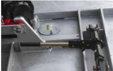
This unit is equipped with a 16,000 lb leveling ratchet jack.
