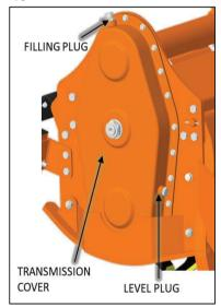
Check the oil level every 50 hours, making sure it reaches the level plug on the transmission cover. If the oil is below this level, fill up oil till restore the level.
