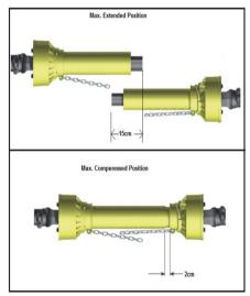
A driveshaft too long may cause structural damages to the tractor and machine. If the driveshaft is too long, it may be adapted by removing it and shortening the tubes according to the instructions provided by the Manufacturer in its use and maintenance manual.
